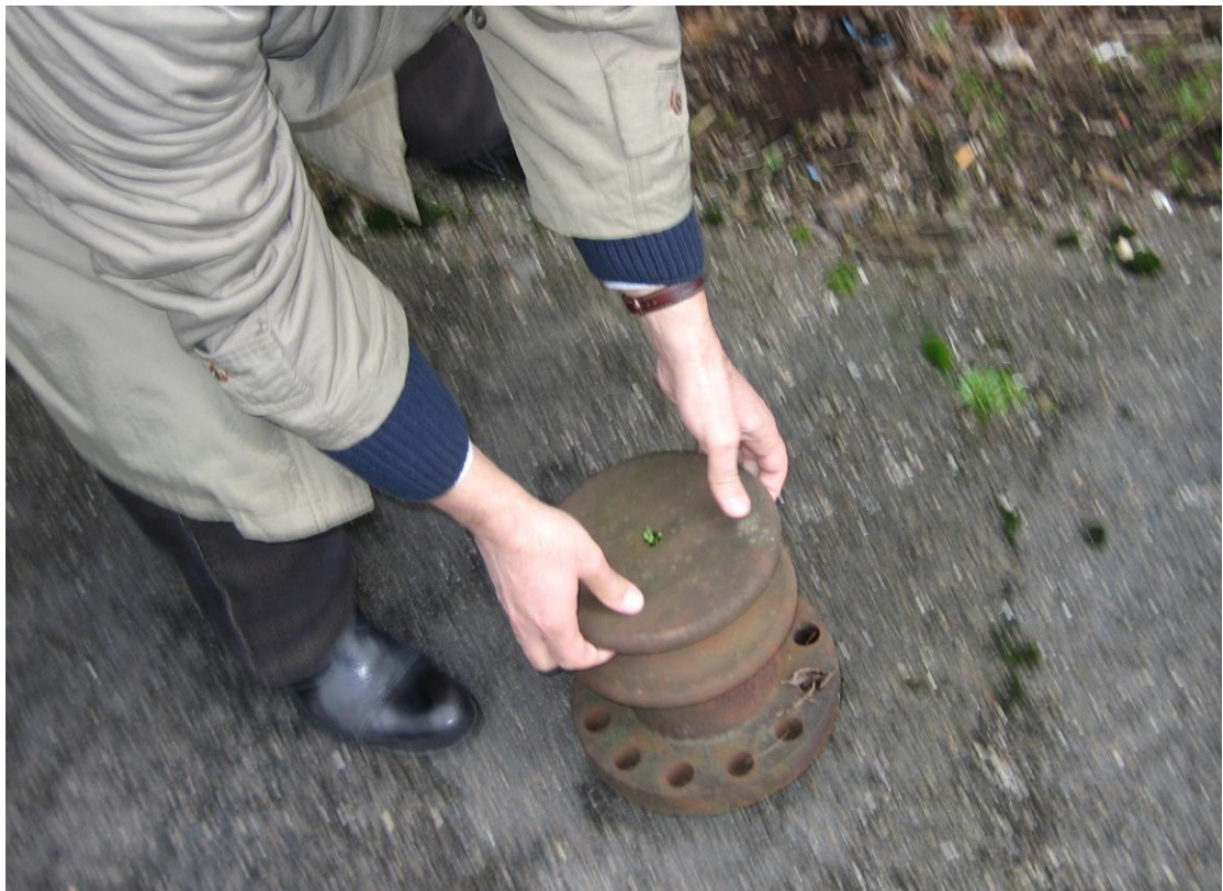
Example of fasteners to be mounted on the magnets
