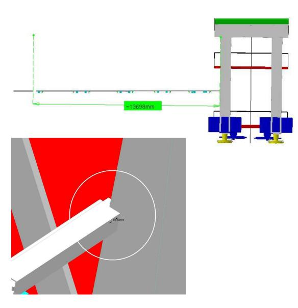
AT612302MQ - BOC Rail Feet, SECTOR 13 VHB\_0001 - CENTRAL PAIR OF FEET B Clash -2 mm Relevant
