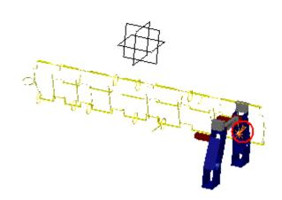
Tomas: Inaccurate design position of cable tray
