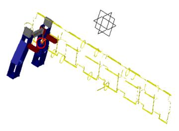
Tomas: Inaccurate design position of cable tray
